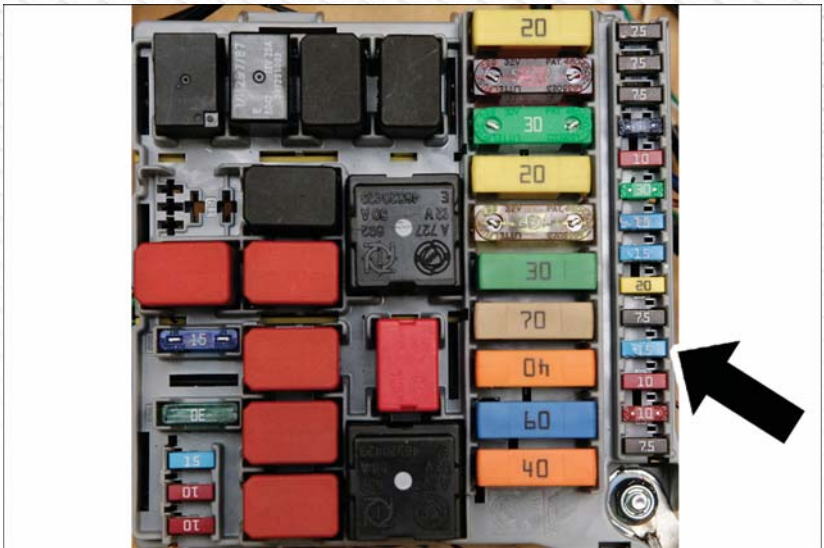
F15 fuse 15 Amp Blue Cigar/Power Outlet Front Console
