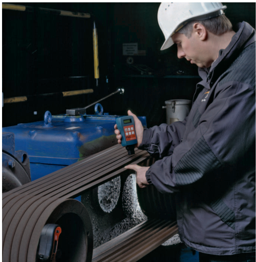
Measurement using cableless measurement probe
