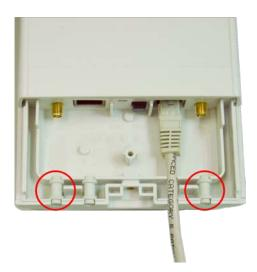
2. Connect your external antenna to the SMA-type connectors at the bottom of the CPE.
