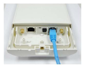
Figure 4 Cable Connection
