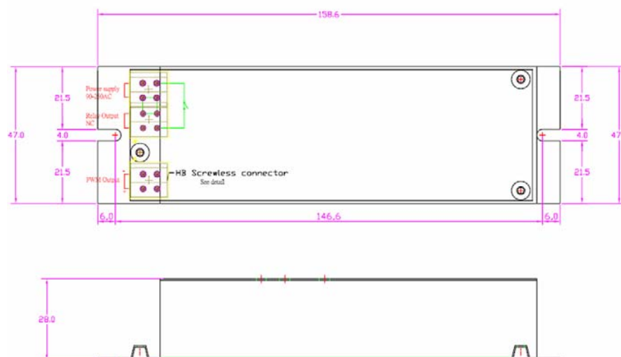
Figure 3.5 Device dimensions without plug-screw clamps
