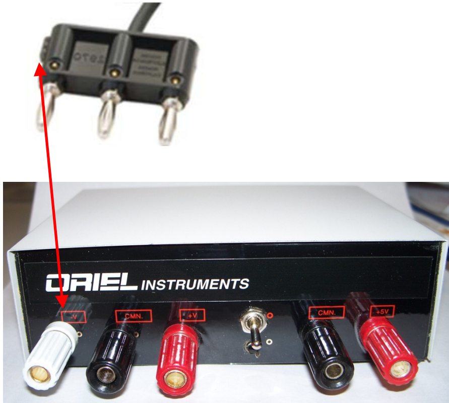
Stand-Alone Preamplifier Power Supply Connection (Si, Ge, Pyro Detectors)
