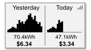
The graphs show hourly data, with a bar for each hour. The height of the bars is proportional to the number of kWh consumed for each hour. The graphs are auto-scaling, and meant to show relative, rather than absolute values.
