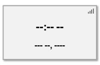
As soon as the dashes are replaced with the current time and date, it means that your **EMU-2**<sup>™</sup> has successfully read the meter, and is ready for use.
