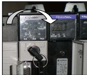
Each time you want to download an application you have to put on “Prog” position (right side). Now you can process to the downloading operation: Go on the menu Communications / Enter on Line / Load
