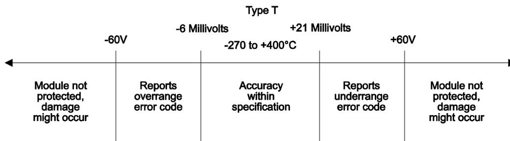
**Figure 1.6 Effect of Voltage Input on Type T Thermocouple**
