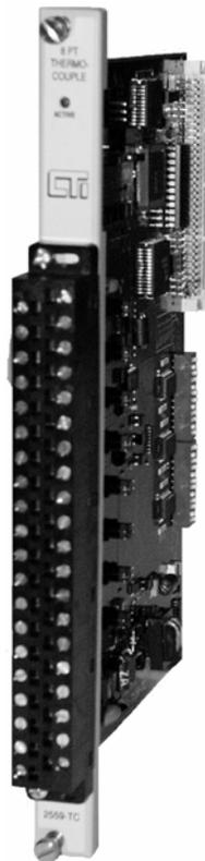
**The Model 2559-TC 8-Pt Thermocouple Module**
