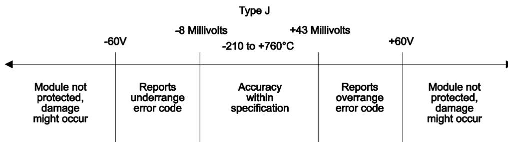
**Figure 1.4 Effect of Voltage Input on Type J Thermocouple**
