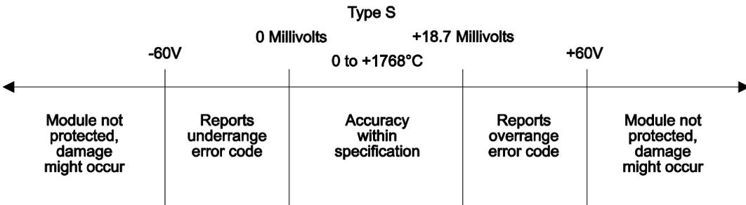
**Figure 1.9 Effect of Voltage Input on Type S Thermocouple**
