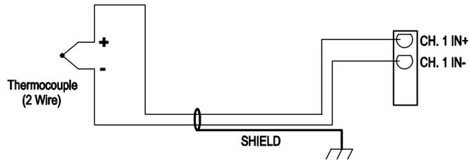
Figure 2.4 Thermocouple wiring application
