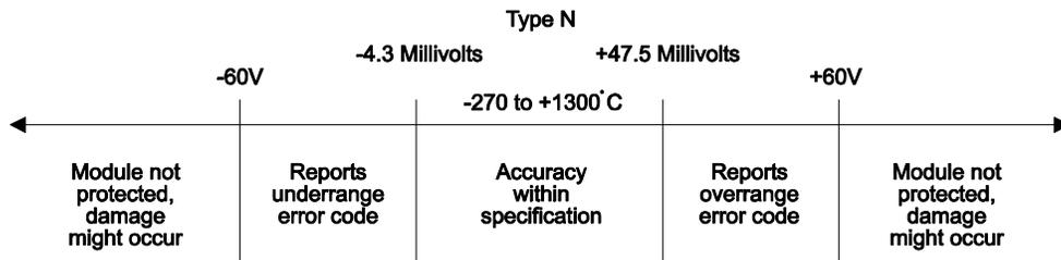
**Figure 1.10 Effect of Voltage Input on Type N Thermocouple**
