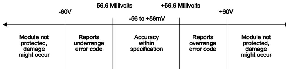
Figure 1.11 Effect of Voltage Input on Type mV Input
