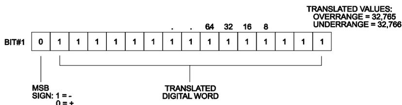
Figure 1.2 Word Input to the PLC from the Module
