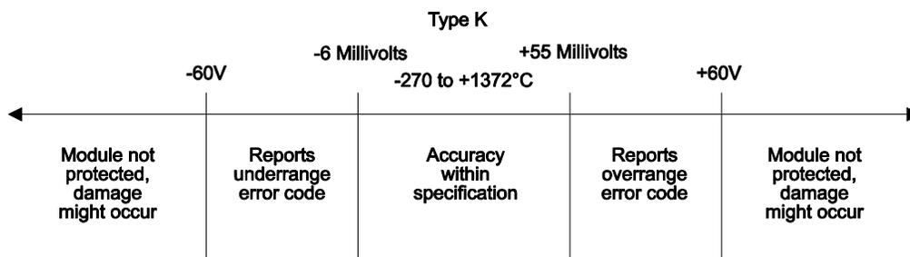
**Figure 1.5 Effect of Voltage Input on Type K Thermocouple**
