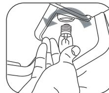
**Warning !** : Disconnect power supply before replacing the lamp.
