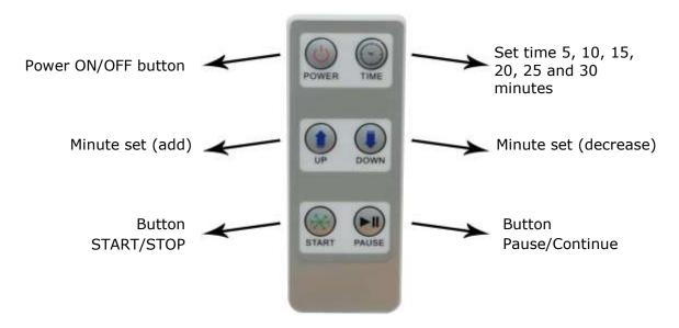
Remark: Remote control effective distance within 5 meters, receive angle about  $45^{\circ}$  degrees.
