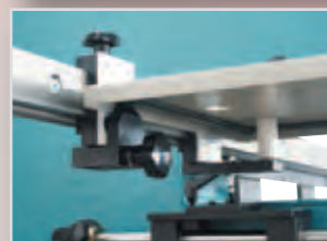
Mutual quick clamping system for selective folding up or down
