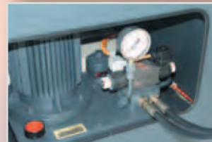
Two circuit hydraulic unit in cabinet base
