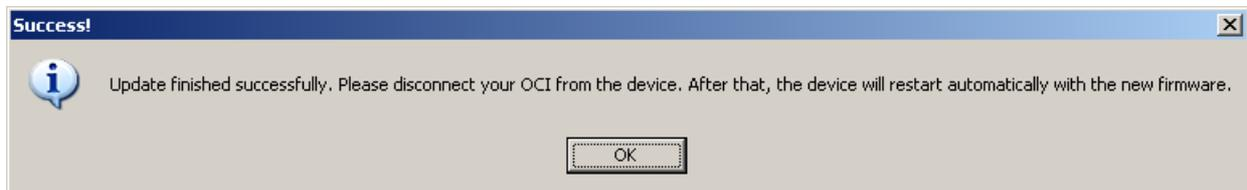
Disconnect the OCI FU cable from the BU. The device will now restart with the new software.
