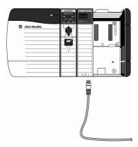
3 Temporarily change the IP address and Subnet Mask on your PC to match the network configuration on the module:
