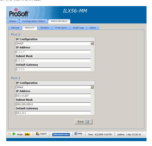
The module has two RJ45 Ethernet ports, located at the bottom of the front panel on the module. You can configure the following settings for each port.
