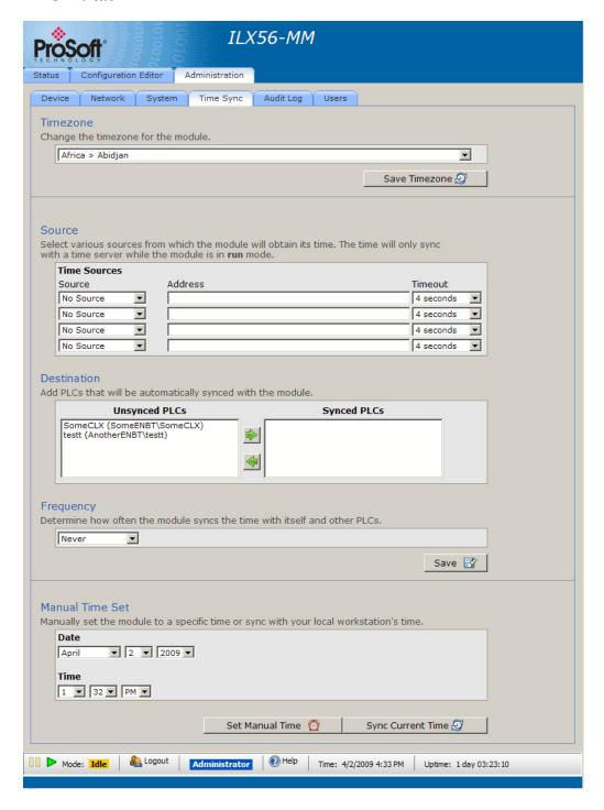
The ILX56-MM module can acquire a time signal from an SNTP time server on the Internet, or from the ControlLogix processor in the same rack with the ILX56-MM.
