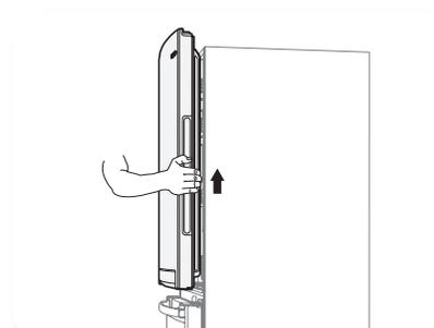
6. Remove the fridge door by lifting it upward.
