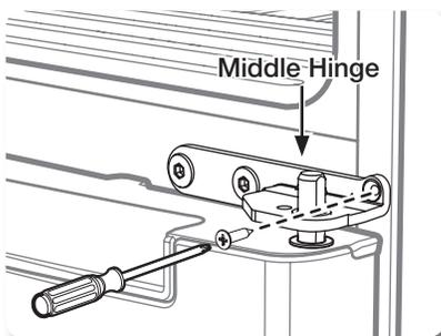
2. After removing one screw and two bolts, remove the Middle Hinge. (Unscrew the screws with the screwdriver(+) and hex bolts with the 4.75mm hex wrench.)
