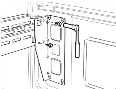
4. With the 10mm wrench, remove two bolts connecting the rail with the door.
