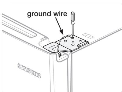
4. Remove the screw that holds the ground wire.
