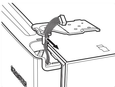
5. Separate Hinge from electric wire and ground wire as shown above.
