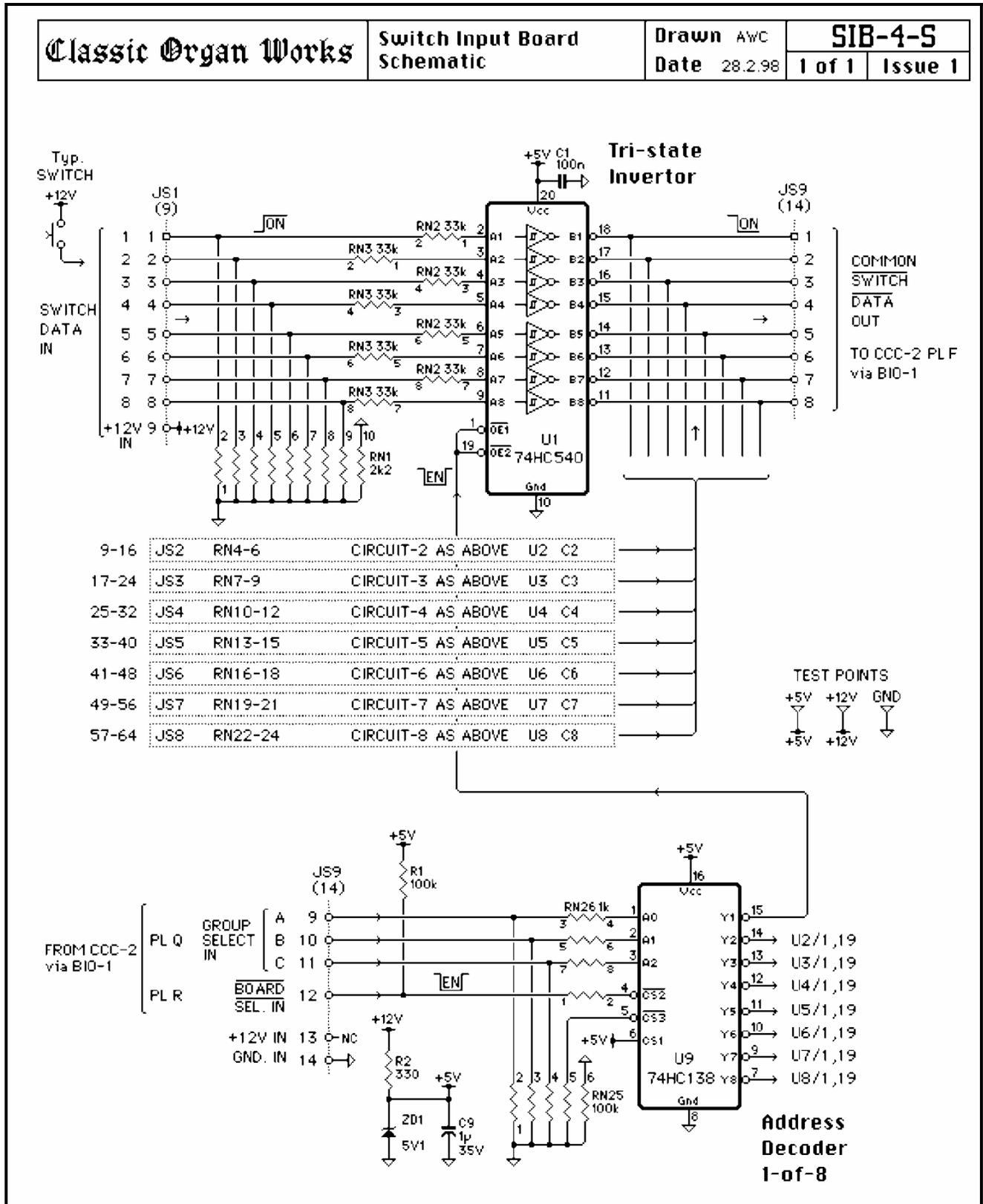
Figure 19: SIB-4 Schematic
