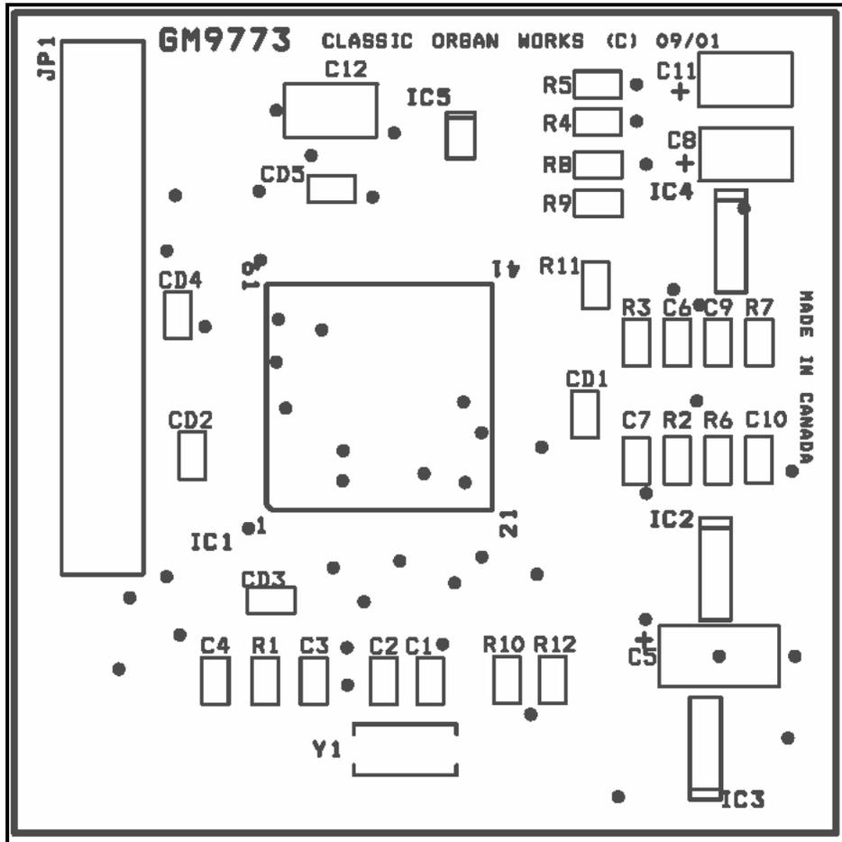
Figure 20: GM9773 Circuit Board Layout
