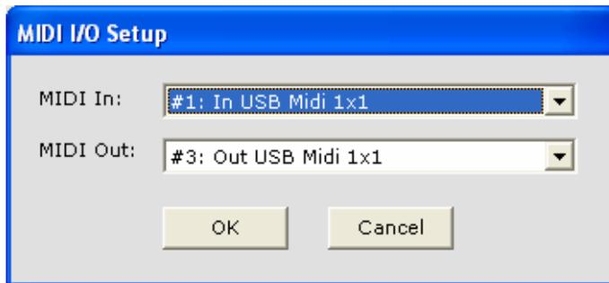
Each of the boxes has a pull-down selection from which you can select a suitable interface device if you have the necessary driver file installed. The one shown is for the M-Audio MIDIspport 1x1, which is a 1-In, 1-Out, USB-to-MIDI converter:
