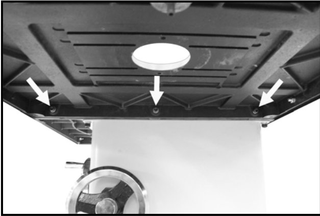
Figure-2 Router table mounted to the saw table
