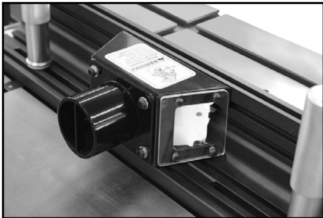
Figure-10 Installing the dust port
