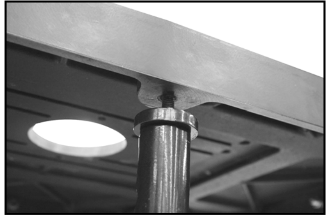
Figure-4 Attaching the support leg to the router table
