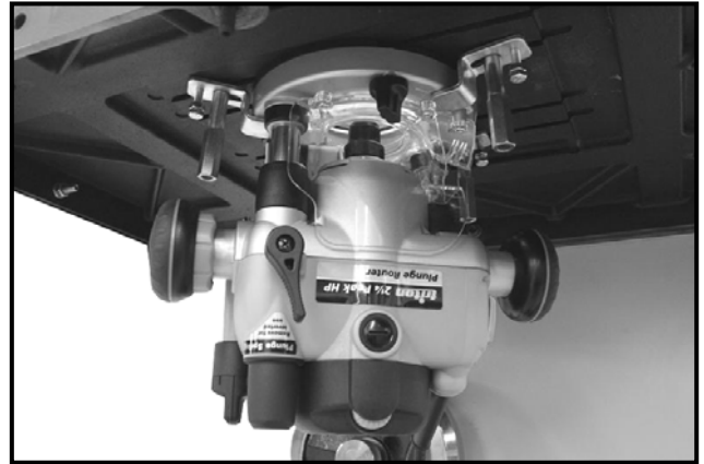
Figure-15 Securing the router to the router table
