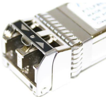
Figure 12a: SFP+ latch closed
