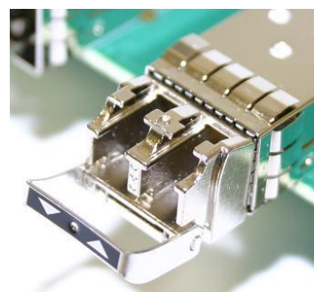
Figure 12b: SFP+ latch open
