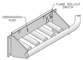
Figure 2: Flame Rollout Switch
