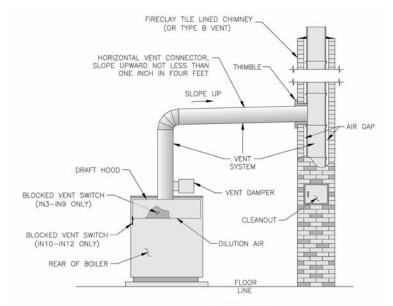
Figure 7: Typical Vent System Installation
