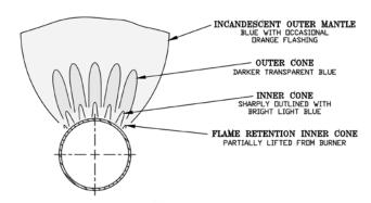
Figure 11: 40mm Main Burner Flame
