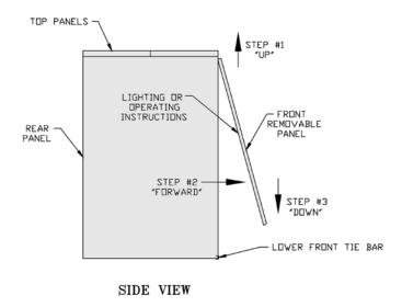
Figure 3: Jacket Front Panel Removal
