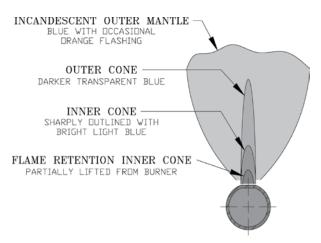
Figure 10: 1 Inch Main Burner Flame
