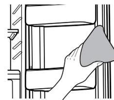
**CAUTION** Do not spray the Refrigerator with water while it is plugged in, as it may cause an electric shock. Do not clean the Refrigerator with benzene, thinner or car detergent due to risk of fire.
