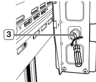
3. Find the best level to align the door slope.
