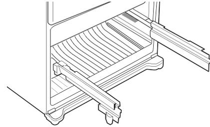
2. Hang the freezer door front onto open slots on the sides.
