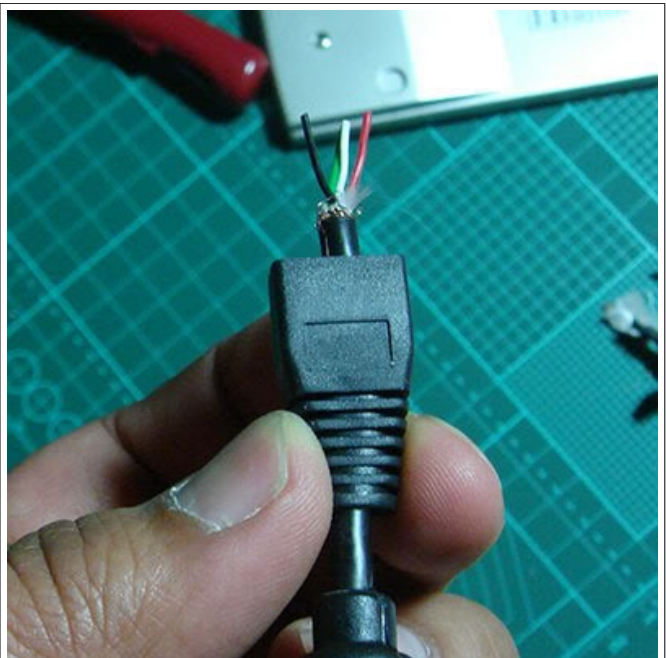
Trimmed cable with boot slid on.
