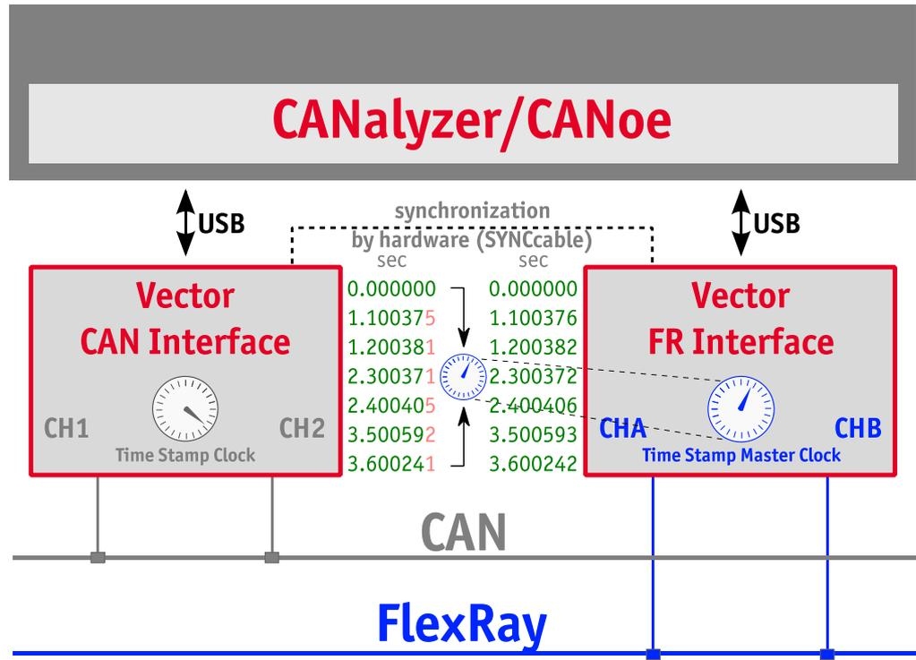
Figure 21: Time stamps are synchronized to the master clock (accuracy in range of 1  $\mu$ s)
