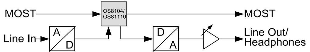
Figure 6: Scheme of line in and line out
