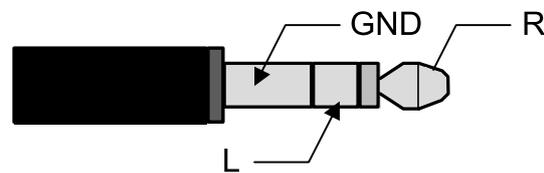
Figure 7: Signal assignment on the stereo jack
