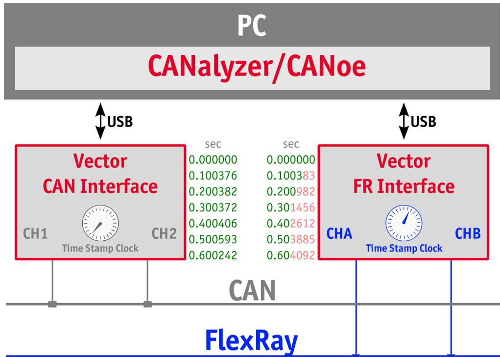
Figure 16: Example of unsynchronized network interfaces. Independent time stamps drift apart
