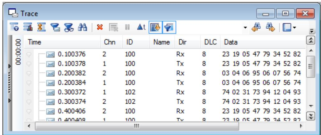
Figure 14: Time stamps of two CAN channels in CANalyzer
