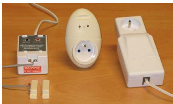
Figure 5: CSH door controller, door sensor, radio controller and X10 controller
