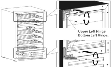
7. Rotate the door  $180^{\circ}$  so that the top is now the bottom, and install it by attaching the support rod with screws.
