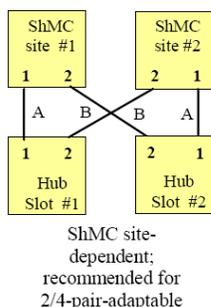
The shelf manager Ethernet ports in a Schroff shelf are wired according to the ATCA site-dependent diagram at the left. If only a single switch blade is installed in slot #1, and a shelf manager switchover occurs, shelf manager #2 will not have network connectivity because its port #1 is wired to Hub slot #2 and port #2 is not used in the default configuration.
