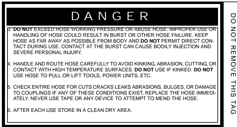
Figure 3-3. Tag attached to “Certified Non-Conductive” hose (front and back).
