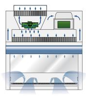
**1A:** Under normal operation with both fans operating (1a) the supply fan creates a negative pressure surrounding the contaminated positive pressure plenum and pushes air across the supply and exhaust filters. The exhaust fan boosts the air pressure through the exhaust filter to create better inflow and operator protection. Supply and exhaust fans automatically operating at reduced speeds extend fan life.
