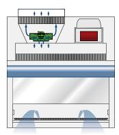
**1B:** If the supply fan fails (1b), downflow to the work area is suspended. The exhaust fan still provide inflow to the cabinet to help maintain containment. The control panel warns of downflow failure.
