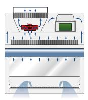
**1C:** If the exhaust fan fails (1c), the supply fan continues to provide inflow to the cabinet and downflow to the work area. The control panel warns of inflow failure.
