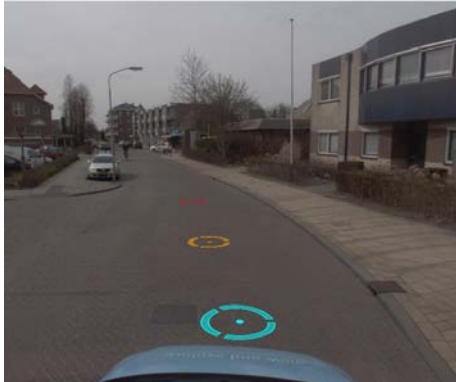
Fig. 97- A changing cursor color indicates the accuracy of measurements possible (The cursor may vary from this image)
