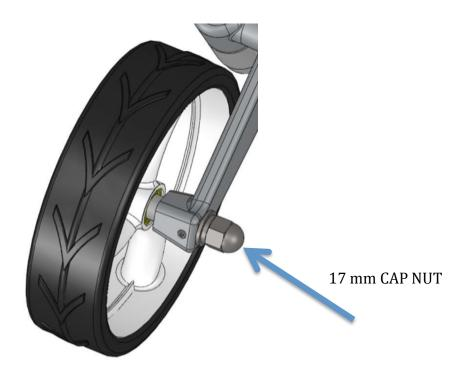
When standing in the front of the trolley looking at the front wheel, loosen the 17 mm nut on the right side of the front wheel.
