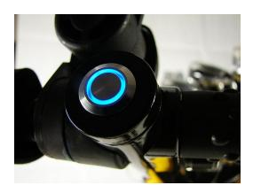
Alternatively, the trolley may be controlled by using the push button at the end of the handle. (Where the blue LED is located). Simply push the button while the trolley is moving and the trolley will stop. The LED will triple flash. Push the button again to resume at the same pace.
