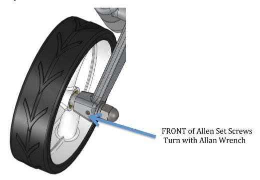
The Allen Set Screws should be gently turned on both the front and back sides an equal amount.
