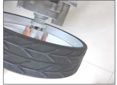
• Install front wheel. Review the following drawing and install the front wheel.
