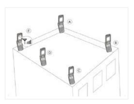
The repeater's main function is to improve weak RF signals in an area. The formula is: Input power + Gain= Output power. The signal strength from an outdoor antenna directly affects the efficiency of the indoor coverage. It is very important to choose the correct outdoor antenna location in order to get the best signal.
