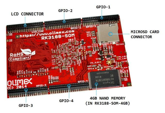
GPIO-1, GPIO-2, GPIO-3, GPIO-4, and LCD\_CON are female connectors with 0.01" step. They are used to attach RK3188-SOM to RK3188-SOM-EVB (or to your custom shield of peripherals).
