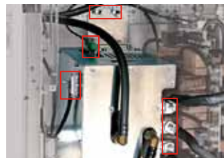
Modules (filter unit and power element) can be released from the front with just a few bolt/plug connections.
