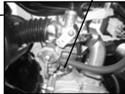
Before transporting the ATV make sure the fuel valve is turned to the off position then drain fuel from the carburetor as follows:
