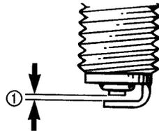
To maintain a proper functioning spark plug, keep the plug free of carbon. Remove carbon from the plug with a wire or pin, and adjust the gap to 0.24 - 0.28 inch (0.6~0.7mm) for good ignition. Use a thickness gauge to check the gap.
