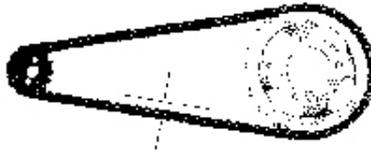
The drive chain should be adjusted and make sure there is 20~30 mm (0.8~1.2 inches) of slack, as shown above.
