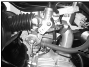
Inspect the fuel hose for damage and fuel leakage. If any defects are found, the fuel hose must be replaced.
