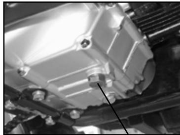
3. Remove the drain bolt and drain oil into proper container.
