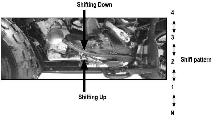
**NOTE:** Only shift to low speed gears when you feel that there is insufficient power to climb hills or continue forward.
