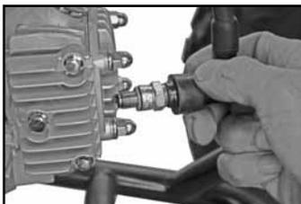
1. Remove the spark plug and reattach it to the spark plug lead.
