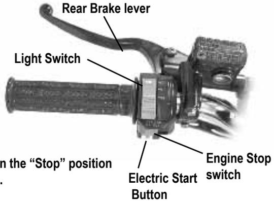
With the Engine stop switch in the “Stop” position
