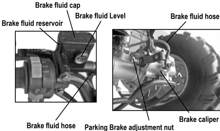
1. Inspect the rear disk brake caliper and brake fluid reservoir for leakage. If brake fluid leaks, the safety of riding could be affected.
