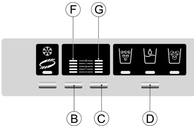
To adjust the refrigerator temperature, press button C. The indicator (G) will illuminate. Each subsequent press of button C will adjust the temperature scale by one. To clear the setting, simply keep pressing button C until indicator (G) is back to level 1.
