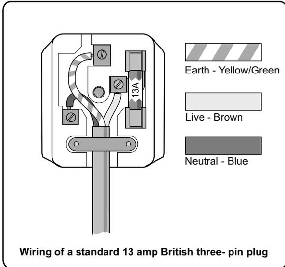
The wire coloured green and yellow must be connected to terminal marked with the letter E, coloured green and yellow or marked with the earth symbol:
