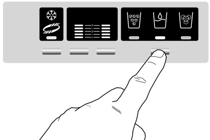
To reset the display, press and hold drinks dispenser button for 5 seconds. The warning will deactivate and the display light will return to blue.
