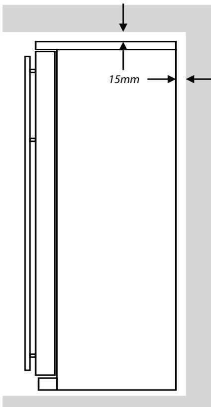
If located close to a corner adequate spacing must be left for door opening and removal of shelves. Refer to diagram.
