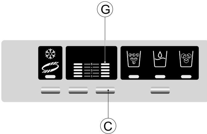
To switch off the refrigerator, press and hold button C for a few seconds. The icon (G) will disappear.
