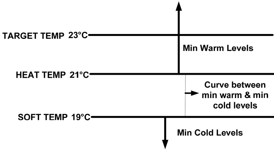
If the inside temperature is above 21°C (heat temperature) the controller will operate according to the Min Warm levels.
