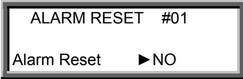
**\*<Note>** To reset the alarm press Enter and use the Round Arrows key to change from NO to YES.
