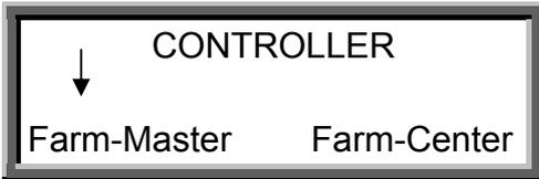
Use the arrow keys to switch between controllers and press select to view the software version.
