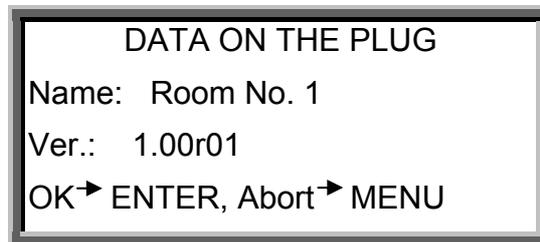
Before loading the setting, you can view setting name and software version for this setting. Press enter to load the data on the controller. To cancel reading from this setting, press MENU.
