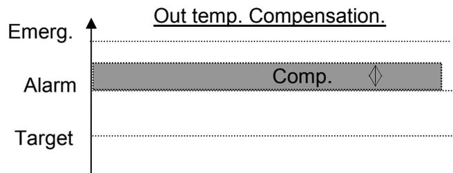
**Emergency Temp.:** The temperature beyond which the controller goes into emergency mode and an alarm is activated.
