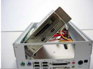
Step 8: Plug the DC12V connector into 1394 card
