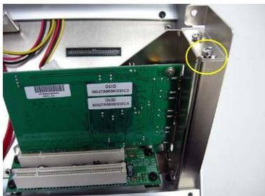
Step 6: Insert your PCI card into the PCI Bus until it is completely seated.
