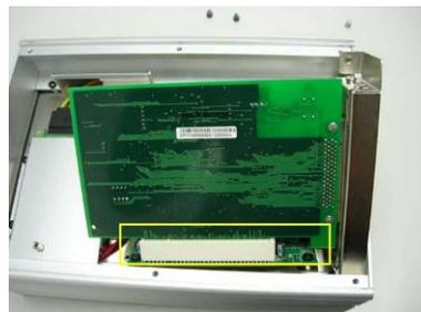
Step 7: Make sure the PCI card install correctly and then fasten the screws of the bracket securely.
