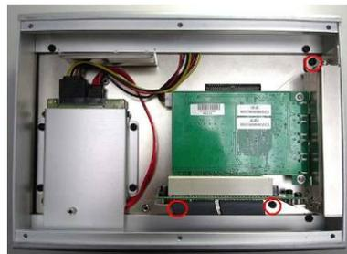
Step 5: Let the PCI bus triangle stand straight up and unscrew the bracket.
