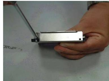
Step 5-1 (for VB-115): Plug the HDD cable adaptor to the back of the 2.5" HDD. The IDE cable will be marked down one side with a red strip, this denotes Pin 1, match this with the Pin 1 indicator on the back of the hard drive.
