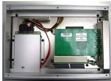
Step 3: Pull out DC12V connector of 1394 card.
