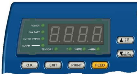
Figure 3: Vision Temperature Recorder - Display Area
