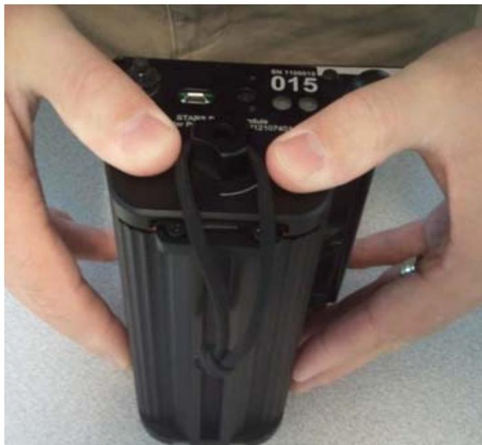
2. Turn on the Sensor Node by pressing the black button on top of the Sensor Node. A single click is all that is needed.
