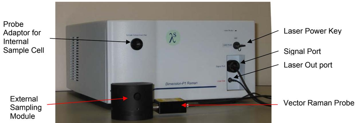
1. Connect the thin black Laser Fiber to the **Laser Out** port, and the Fiber Slit Assembly end of the thick black Signal Fiber to the **Signal Port** on the lower right front panel of Dimension-P1 Raman.
