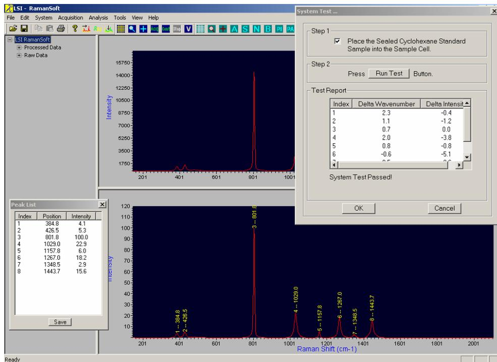
If the system test is passed, click *OK* to continue the tour. If the test fails, a re-calibration of the instrument is then necessary. Please refer to section “Calibration” of Chapter 5, “RamanSoft Basic Functionalities”, to re-calibrate the system.
