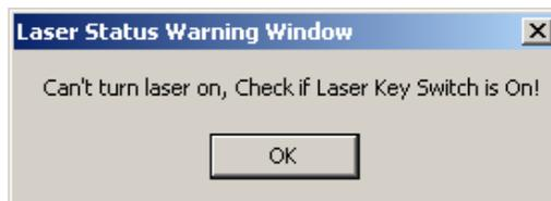
The warning indicates that the laser is not turned on yet, i.e., the Laser Power key is at OFF position (on the front panel of the Dimension-P Raman).
