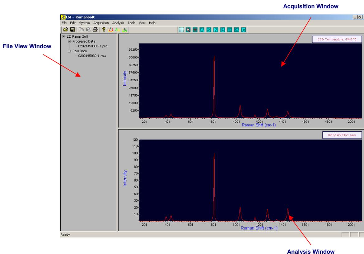
The Acquisition Window displays the acquired raw spectrum (of cyclohexane), the Analysis Window displays the processed spectrum (here the background-removed and normalized cyclohexane spectrum – see later sections on RamanSoft Data Processing methods), and the File View Window displays *Raw Data* files and the *Processed Data* files for the current RamanSoft session. Double clicking any of these files places that raw or processed spectrum in the Analysis Window.
