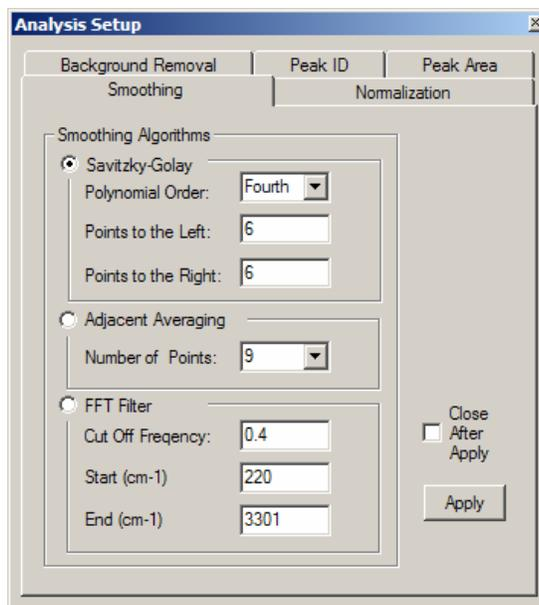
For applying S-G smoothing on Raman peaks, a *Polynomial Order* of 4, and both the number of *Points to the Left* and number of *Points to the Right* of 6 are recommended to maintain the original peak shape.
