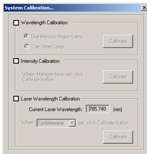
System calibration is performed with the LSI Calibration Kit. To do this, the user needs to insert the Vector Raman Probe into the LSI Calibration Kit as shown below, turn the adjustable aperture to allow highest (but not saturated) signal intensity.
