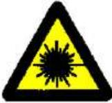
**Caution!** The use of this symbol on equipment indicates that the laser should not be operated without first consulting the manual. The same symbol appears in the manual adjacent to the text that discusses the hardware item(s) in question.
