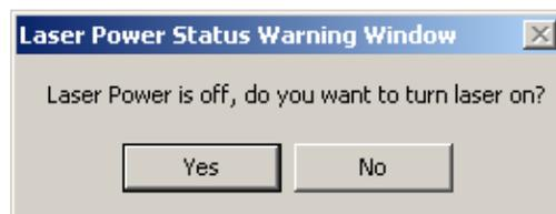
click Yes. Wait till the Laser Power Stabilizing Window disappears. Note that this window sometimes appears as the system automatically turns off the laser if the system has been idle for more than 30 minutes.
