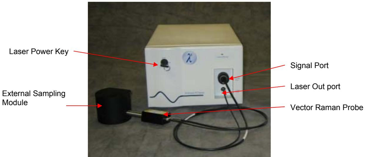
1. Connect the thin black Laser Fiber to the **Laser Out** port, and the Fiber Slit Assembly end of the thick black Signal Fiber to the **Signal Port** on the lower right front panel of Dimension-P2 Raman.
