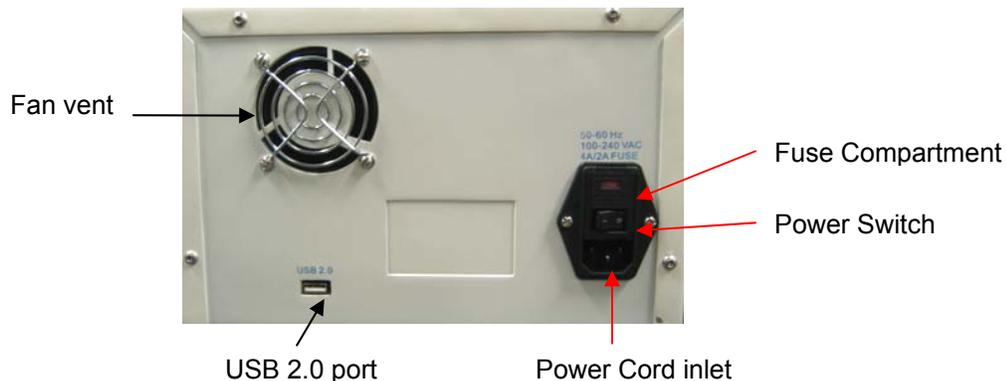
5. Plug in the power cord of the Dimension-P2 Raman and of the computer, respectively.
