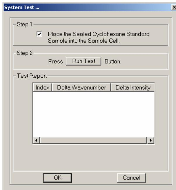
Press *Run Test*. The system starts to acquire the spectrum for the sealed cyclohexane standard sample, and the test results appear in the *Test Report* group box of the System Test widow.
