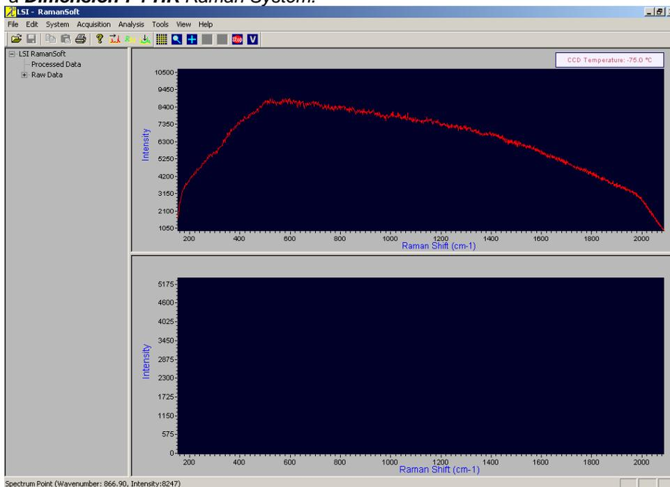
The LS-1-Cal (Ocean Optics, Inc.) calibration lamp spectrum on a **Dimension-P1 SR** Raman System.
