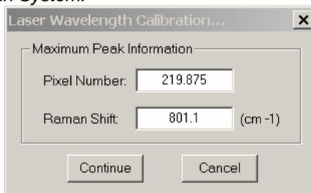
5. Click on *Continue* button once the user has confirmed the *Pixel Number* reading of the maximum cyclohexane peak, RamanSoft will then perform the laser wavelength calibration.
