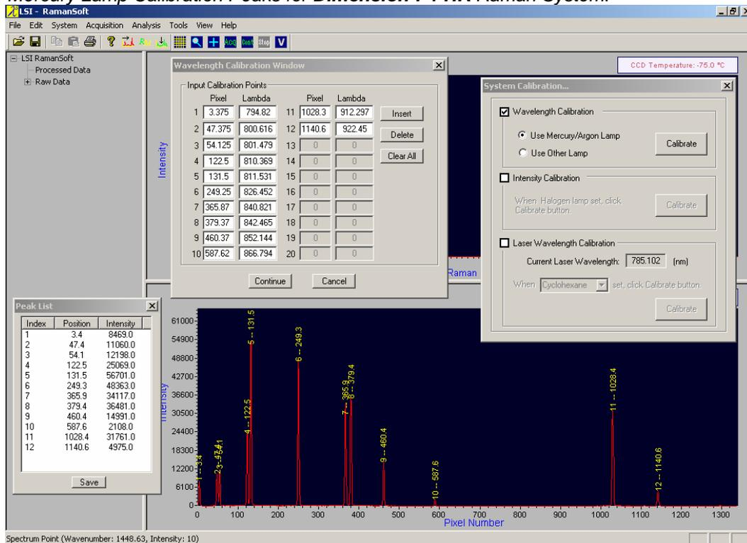
For Dimension-P1 high resolution (HR) models, the program uses 12 standard Mercury/Argon peaks (as labeled in the above figure and tabulated in the Wavelength Calibration Window below) to perform the wavelength calibration (see Appendix II for a full-page view of the above figure where the 12 standard peaks can be clearly discerned, and a table for the mercury/argon lamp peak wavelengths).
