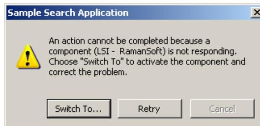
The laser might be off, as the system automatically turns the laser off if there is no acquisition for 30 minutes. Click on *Switch To...* button. The Laser Power Status Warning Window will appear.
