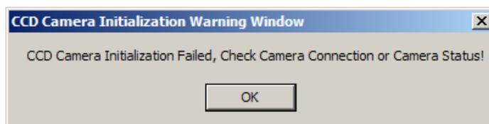
The USB 2.0 cable between the Dimension-P Raman unit and the computer may not be properly connected. Connect the USB 2.0 cable, make sure that the two ends of the USB cable is push-tight, and restart RamanSoft.
