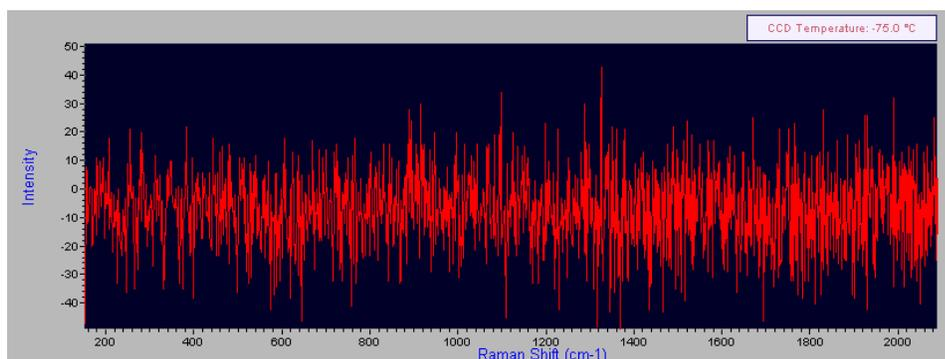
and the sample is placed properly in the internal sample cell or the External Sampling Module and that it is believed to have a Raman signal, the laser might be off (the program turns the laser off automatically if the system has been idle for more than 30 minutes). Go to *System->Laser Setting*, and make sure that *Laser On* is checked. If not, click on *System->Laser Setting->Laser On* to turn the laser on. See the following section “Turn Laser On From RamanSoft” for more details.
