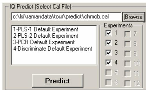
**Note:** The laser may turn off automatically if the system has been idle for more than 30 minutes. Make sure that the laser is on by checking *System->Laser Setting->Laser On* before pressing *Predict*.
