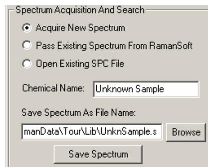
**Note:** The laser may turn off automatically if the system has been idle for more than 30 minutes. Make sure that the laser is on by checking *System->Laser Setting->Laser On* before pressing *Start Search*.
