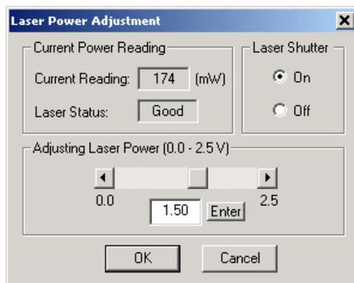
Set the laser power to the desired value (100 – 200 mW is recommended) by dragging the bar in the *Adjusting Laser Power (0.0 – 2.5 V)* group box, or by entering a number between 0 and 2.5 in the text entering box. The adjusted laser power is displayed in the *Current Reading* of *Current Power Reading* group box. Click *OK*.
