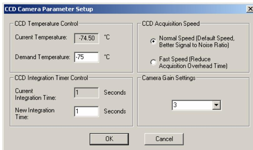
Set the *New Integration Time* to be what is desired (1 second is usually sufficient and recommended for most solid and solvent samples, longer integration time is recommended for aqueous samples). Signal intensity may also be adjusted with the Gain Setting, with 3 yielding the highest signal. Leave *CCD Acquisition Speed* as *Normal Speed* (default).
