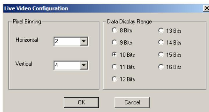
The *Live Video Configuration* menu provides the settings to configure for acquiring and displaying a CCD image. This is an essential tool for a system engineer to adjust alignment of fiber optics in the Raman spectrometer system.
