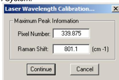
The pixel position and the Raman Shift of the maximum cyclohexane peak identified on a **Dimension-P1 SR Raman System**.
