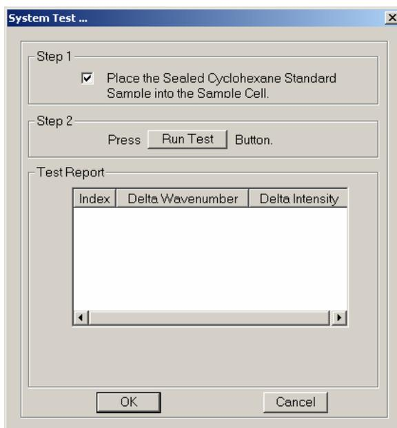
3. Press **Run Test** button in Step 2 group box. The system takes the cyclohexane spectrum, identifies the cyclohexane peaks, and updates the System Test window with test results.
