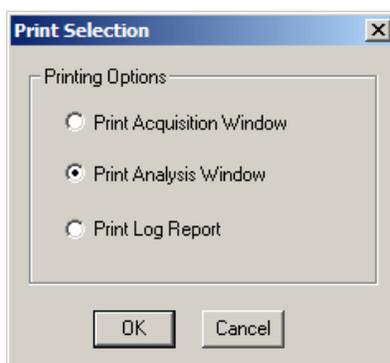
*Print Acquisition Window* allows for printing the spectrum displayed in the Acquisition Window, along with the system parameters and file information such as CCD temperature, CCD integration time, date/time, file name and path, operator name, sample name/info.
