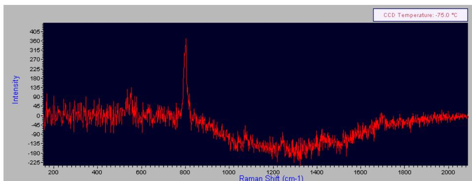
For the user's comparison, the original spectrum (10% aqueous acetone in glass vial) prior to background subtraction is shown in the following figure. In the above figure, the dip between 1000 – 1600  $\text{cm}^{-1}$  could be due to an incomplete match between the measured sample and the background sample.
