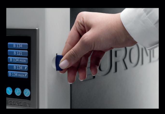
The practical SD card holder, mounted on the side of the new E9 Recorder, allows you to easily transfer sterilisation data from the autoclave and store them on a PC to maintain track of all the operations performed. The new E9 Recorder also has PC serial connection and Ethernet connection ports.
