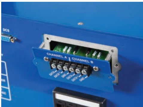
Figure 10.8 - Removing Network Surge Protector
