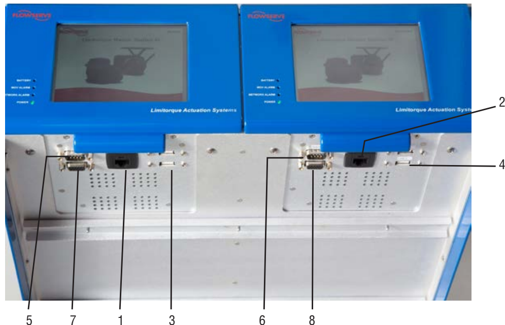
Figure 4.4 - Master Station Front Panel Connections
