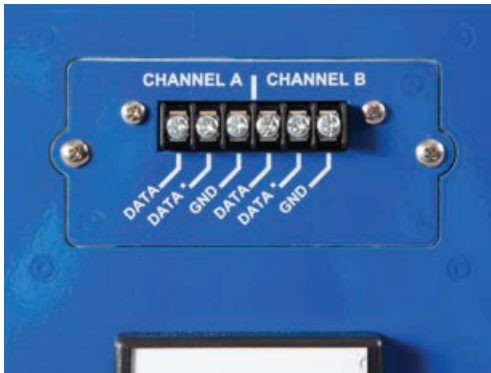
Figure 10.7 - Network Surge Protector
