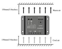
Figure 3-1 Mounting and cooling
