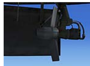
Ram Air Turbine
