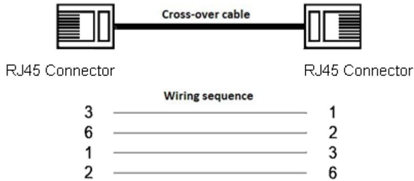
Figure 11 10/100M Cross-over Cable Wiring
