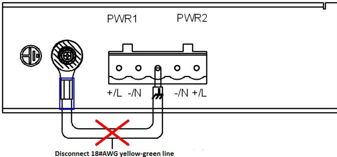
Figure 16 Disconnect 18#AWG Yellow-green Line
