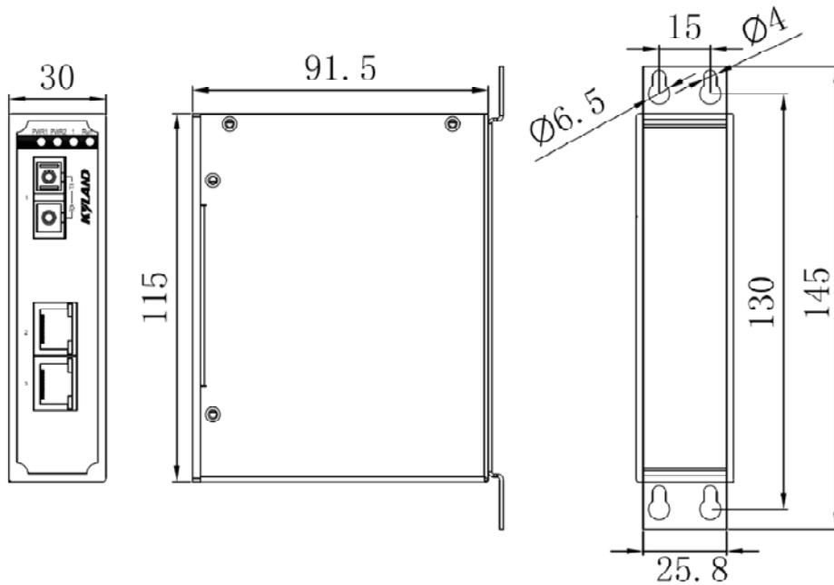
Figure 4 Panel Mounting Dimension Drawing
