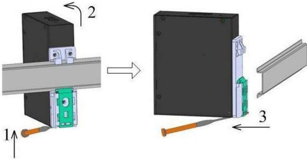
Figure 6 DIN-Rail Dismounting
