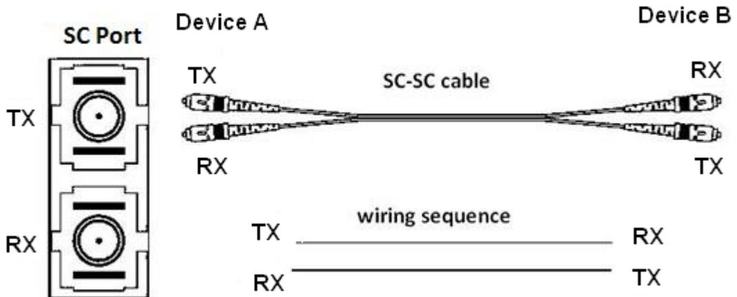
Figure 12 100Base-FX Port Wiring
