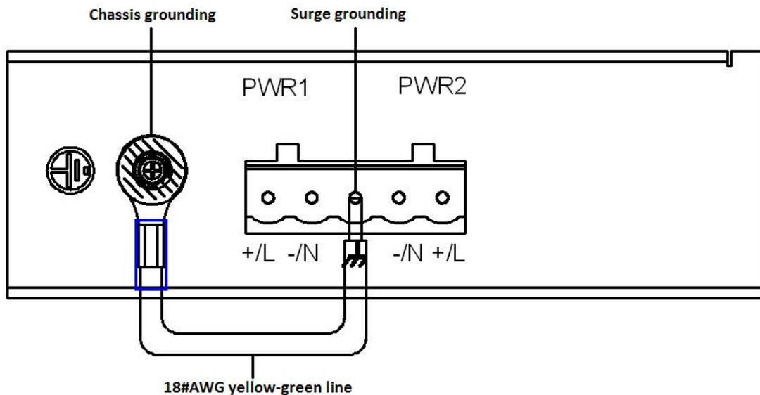
Figure 14 Chassis Grounding and Power Terminal Grounding
