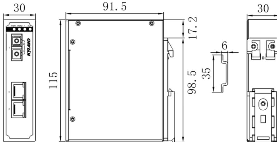
Figure 3 DIN-Rail Mounting Dimension Drawing
