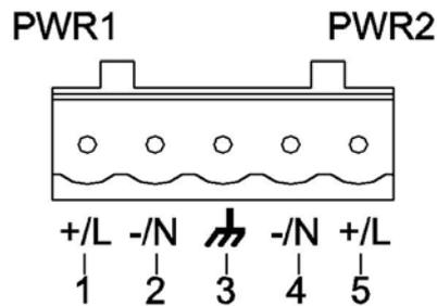
Figure 13 5-pin 5.08mm-spacing Plug-in Terminal Block
