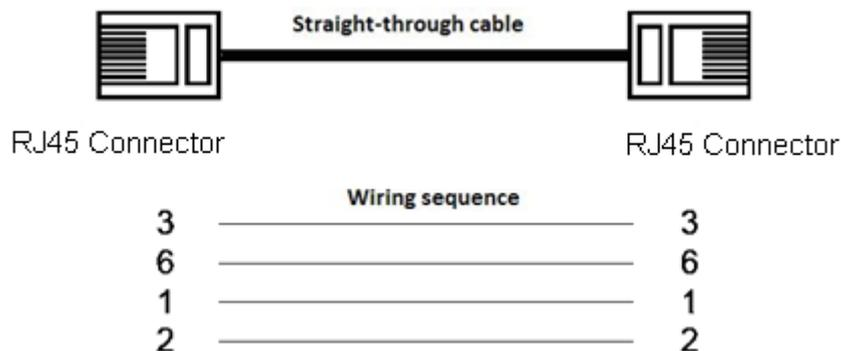
Figure 10 10/100M Straight-through Cable Wiring
