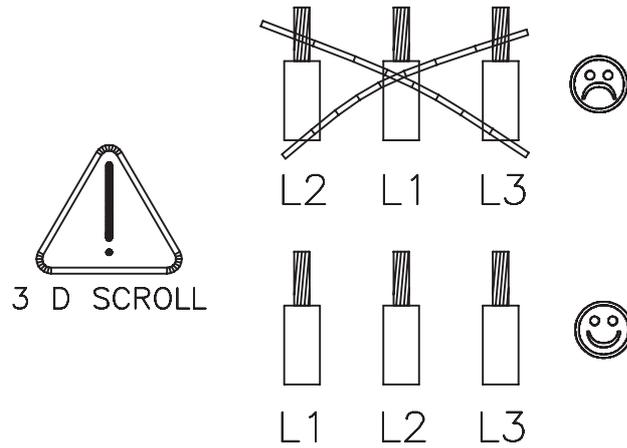
**Note** Make sure phase order is correct. Should the compressor be noisy, reverse 2 phases.
