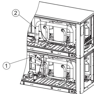
1 = Connection for pressure relief valve circuit 1
