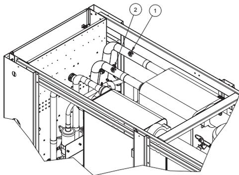
1 = Connection for pressure relief valve circuit 1
