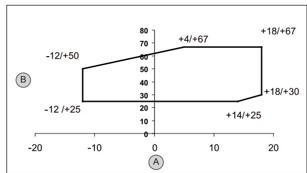
A = Evaporator leaving water temperature (°C)
