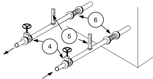
**Figure 12 - Connection of units without hydraulic module - Evaporator and condenser sides**
