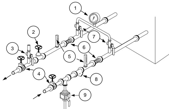
1 = Pressure gauges: show entering and leaving water pressure (2 pressure ports are available inside of the unit - see item 1 in Figure above)
