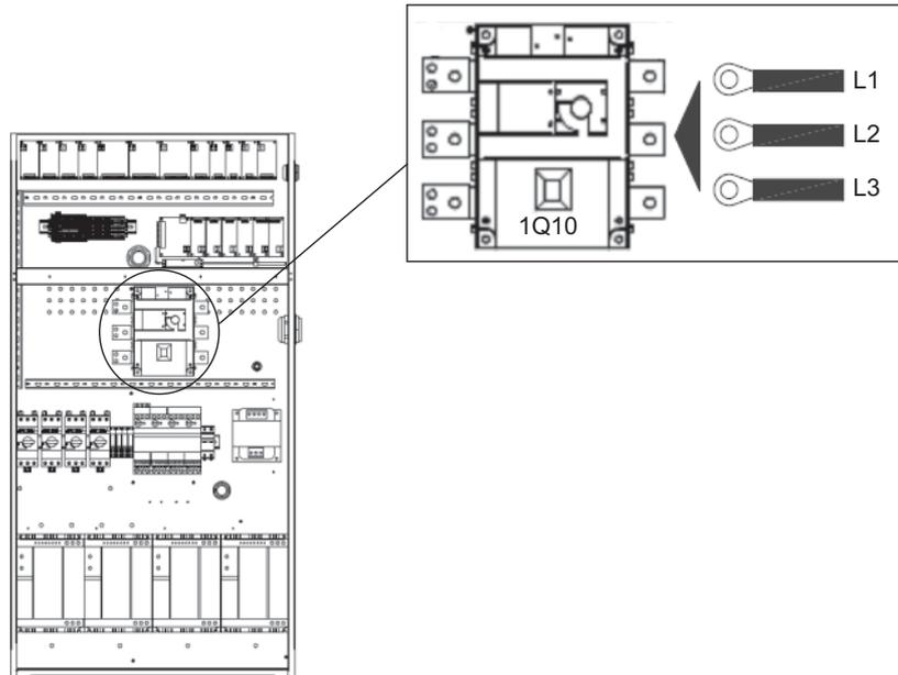
**Figure 23 - CGWN and CCUN main power supply connection (212-215)**
