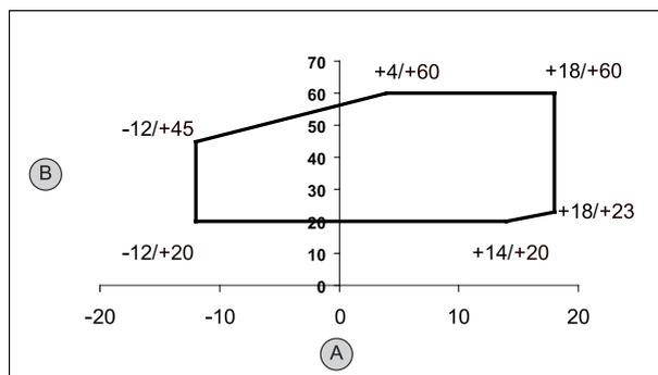
A = Evaporator leaving water temperature (°C)
