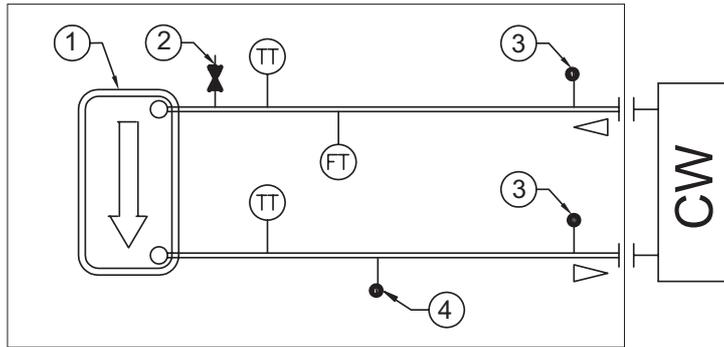
Figure 6 - CCUN hydraulic flow chart - without hydraulic module (212-215)
