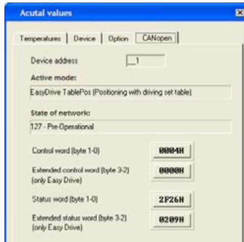
Fig. 6.63 CAN open communication status
