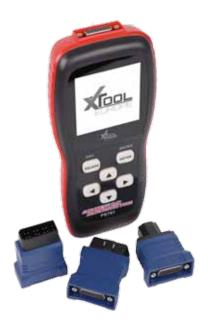
The PS701 has been designed to specifically cater for Japanese vehicles with JOBD and OBDII protocols.
