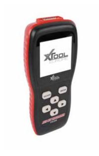
The PS300 is the most comprehensive key programmer in the X Tool range. The handheld device offers key programming; remote programming; PIN code reading and immobiliser unit programming amongst many other features.
