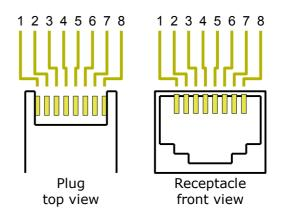
All eight pins are routed between the two connectors. The device doesn't use the unassigned lines.
