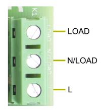
Connect the 230 V or 120 V mains between N/LOAD and L.
