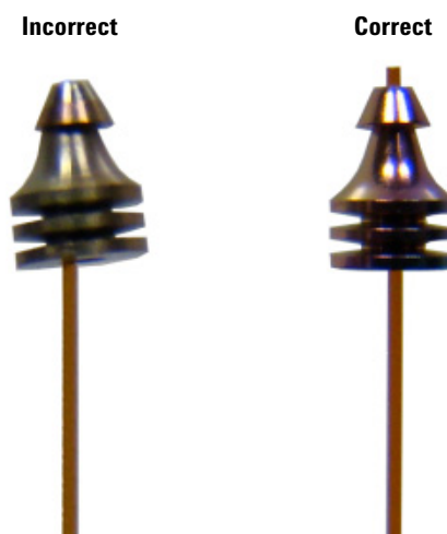
Figure 8 Incorrect and correct swaging symmetry
