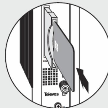
Insert the smartcard completely into the CAM slot. Card contacts looking left and forwards when it is being inserted.
