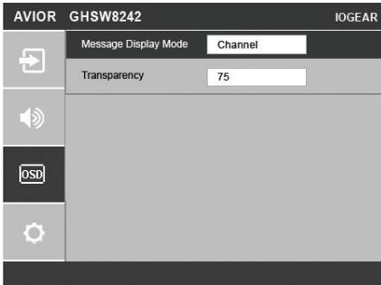
1. Use the drop-down menu to select which display mode the GHSW8242 uses to display information in the upper left corner of the screen. Options are as follows.
